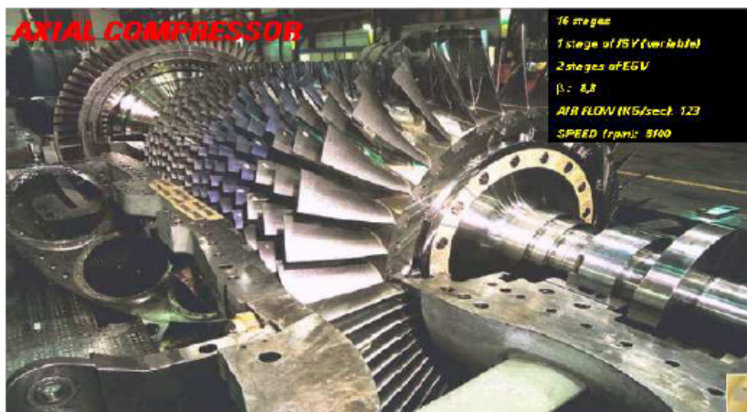
Figure 2.9: aubes du rotor.
