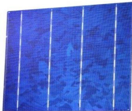
**Figure (I.23) :** Cellules poly-cristallin [43].
